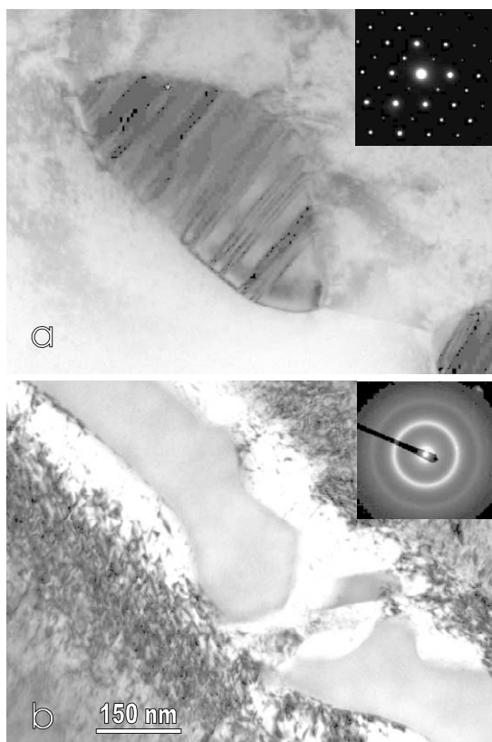
Fig. 4. Micrographs showing precipitates in samples of (a) 0.7 dpa and (b) 3.4 dpa. The diffraction pattern in each graph was taken from the corresponding precipitates. Notice the structure of the precipitates changes from crystalline to amorphous when the dose increases from 0.7 to 3.4 dpa.
